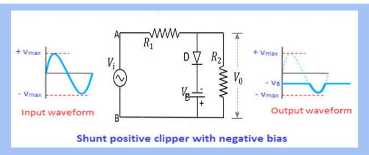
□ **During the positive half cycle**, the diode is forward biased by both input supply voltage V<sub>i</sub> and battery voltage V<sub>B</sub>. Therefore, no signal appears at the output during the positive half cycle.
