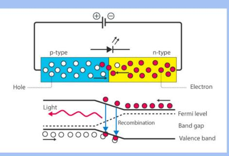
The recombination indicates that the electrons in the conduction band jump down to the valence band. When the electrons jump from one band to another band the electrons will emit the electromagnetic energy in the form of photons and the photon energy is equal to the forbidden energy gap ( $E_g$ ).
