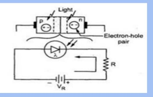
Depletion Region Width: The photodiode is indeed connected in reverse bias to increase the width of the depletion region, enhancing its sensitivity to incident light.
