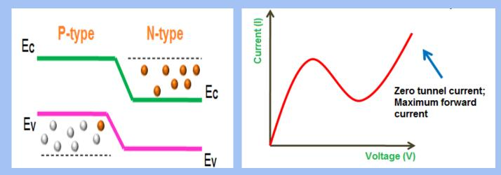
If this applied voltage is greater than the built-in potential of the depletion layer, the regular forward current starts flowing through the tunnel diode.
