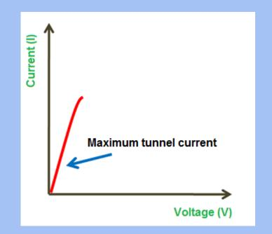
In simple words, the energy level of an n-side conduction band becomes exactly equal to the energy level of a p-side valence band. As a result, maximum tunnel current flows.
