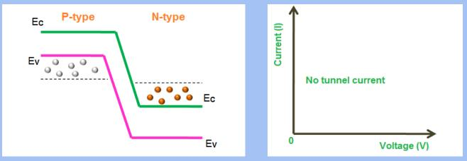
Because of this overlapping, the conduction band electrons at n-side and valence band holes at p-side are nearly at the same energy level. So when the temperature increases, some electrons tunnel from the conduction band of n-region to the valence band of p-region. In a similar way, holes tunnel from the valence band of p-region to the conduction band of n-region.
