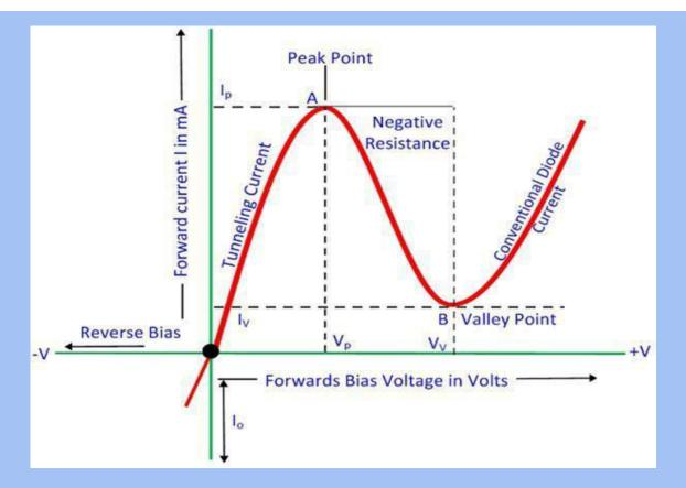
□ In forward biasing, the immediate conduction occurs in the diode because of their heavy doping. The current in a diode reached their maximum value I<sub>P</sub> when the V<sub>p</sub> voltage applied across it. When further the voltage increases, the current across the terminal decreases. And it decreases until it reaches their minimum value. This minimum value of current is called the valley current I<sub>v</sub>.
