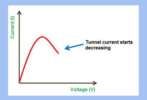
Since the conduction band of the n-type material and the valence band of the p-type material sill overlap. The electrons tunnel from the conduction band of n-region to the valence band of p-region and cause a small current flow. Thus, the tunneling current starts decreasing.
