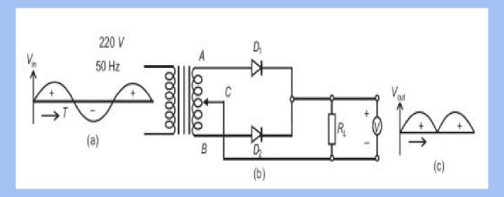
At any moment during a cycle of, V<sub>in</sub> if point A is positive relative to C, point B is negative relative to C. So, the voltage applied to the anode of each diode is equal but opposite in polarity at any given instant.
