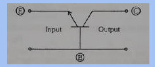
**Current amplification factor** ( $\alpha$ ): It is defined as the ratio of change in collector current to the change in emitter current at constant collector base voltage V<sub>CB</sub>.
