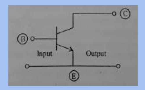
Current amplification factor ( $\beta$ ): It is defined as the change in collector current to the change in base current at constant collector emitter voltage  $V_{CE}$ .
