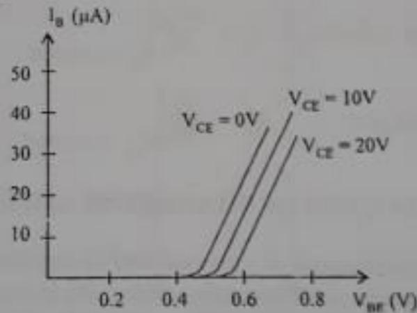
As reverse bias voltage  $V_{CE}$  increases, depletion region in collector base increases. Hence the width of base available for conduction decreases. Hence  $I_B$  decreases due to early effect and graph shift towards X-axis.
