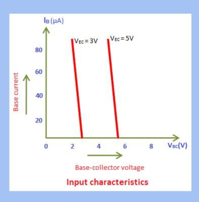
☐ The input characteristics describe the relationship between input current or base current (I<sub>B</sub>) and input voltage or base-collector voltage (V<sub>BC</sub>).
