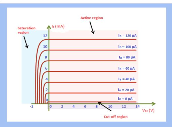
□ The output characteristics describe the relationship between output current or emitter current (I<sub>E</sub>) and output voltage or emitter-collector voltage (V<sub>EC</sub>).
